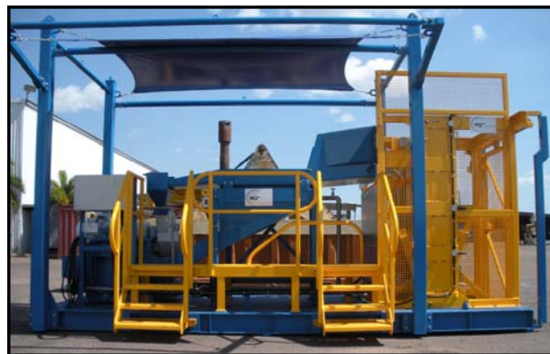
AGR's patented NORM processing plant
